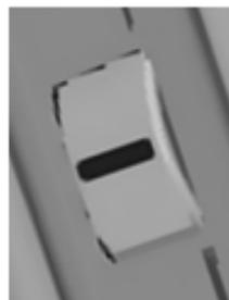
In contrast to conventional hand-held measuring devices, this apparatus has a “THUMB WHEEL” on the left-hand side of the housing. This wheel allows a 15° upward or downward rotary movement, and can also be pressed in the central position.
