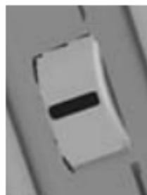
In contrast to conventional hand-held measuring devices, this apparatus has a “THUMB WHEEL” on the left-hand side of the housing. This wheel allows a 15° upward or downward rotary movement, and can also be pressed in the central position.
