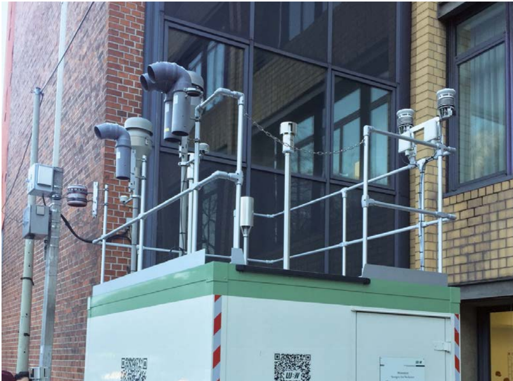
Figure 2.1: Measuring equipment to monitor air quality – here, at the main road Am Neckartor in Stuttgart (Photo: A. Dittler).
